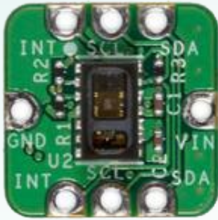
Figure 2: Maxim's popular MAXREFDES117# heart rate module reference design is tiny yet comes equipped with a pulse rate/oximeter sensor, a step-down DC-DC converter, and a logic-level translator
