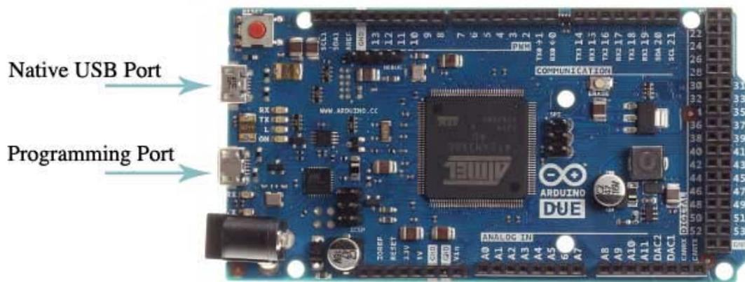
Either of the USB ports can be used for programming the board, though it is recommended to use the Programming port due to the way the erasing of the chip is handled :
