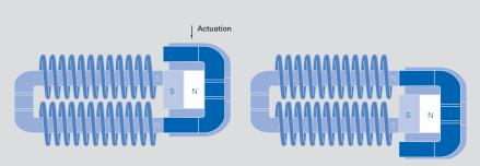
Intelligent energy converter: The inductive generator converts mechanical energy into an electrical energy pulse by continuously changing the direction of the magnetic field.
