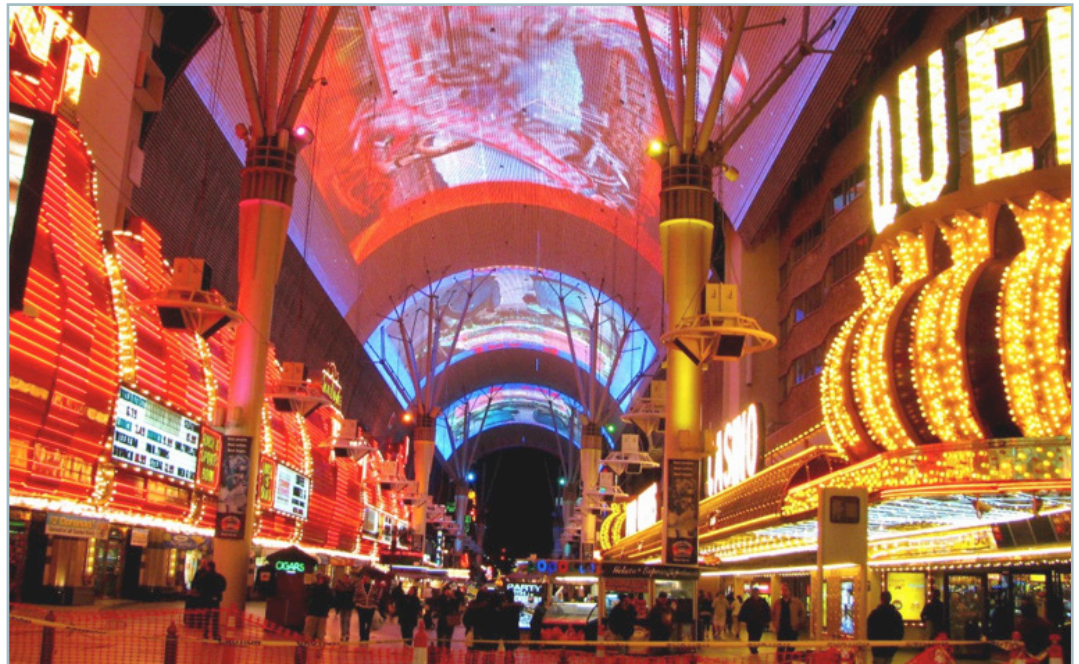
Figure 1: What happens in Vegas... the Fremont Street Experience LED display has 7,552 x 552 pixel resolution with a 2" pixel spacing and consumes 2.2 MW at full brightness. With 12.5 million LEDs, it measures 1,500' x 90' (Image courtesy of Indianapolis Museum of Art)
