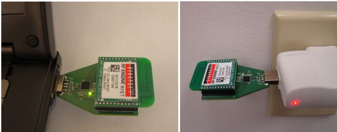
Figure 25 - A SNAPstick drawing power from a laptop PC and USB AC Adapter
