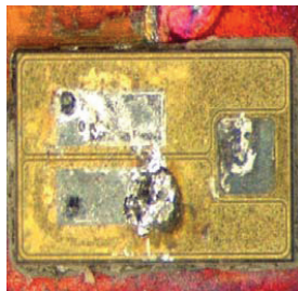
Fig 68. Sample image 5; 15 V, 2.5 A, 100 ms
