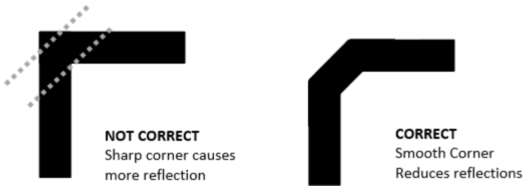
Figure 18. Poor and correct way of bending traces in right angles
