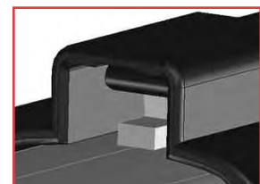
Locking latch shown fully depressed, latch releases locking ramp
