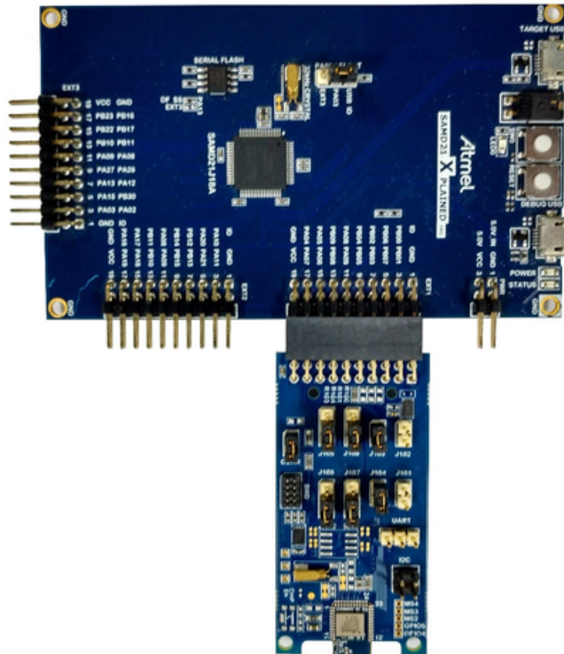
Figure 3-5. ATBTLC1000-ZR Xplained Pro Extension Connected to the SAM D21 Xplained Pro
