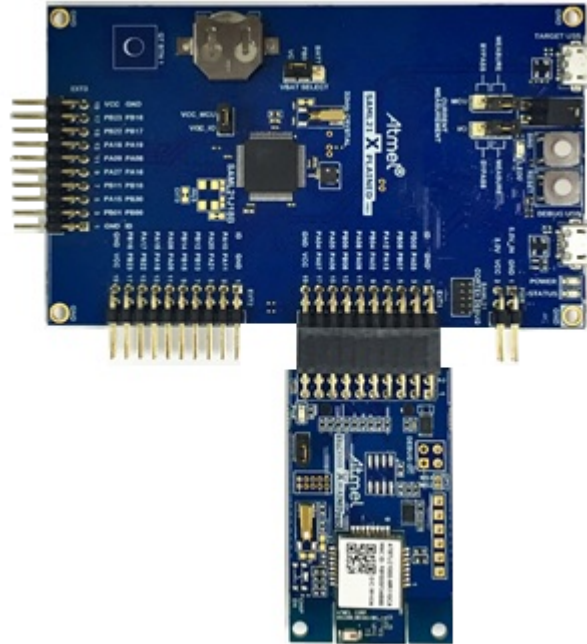
Figure 3-3. ATBTLC1000-MR Xplained Pro Extension Connected to the SAM L21 Xplained Pro
