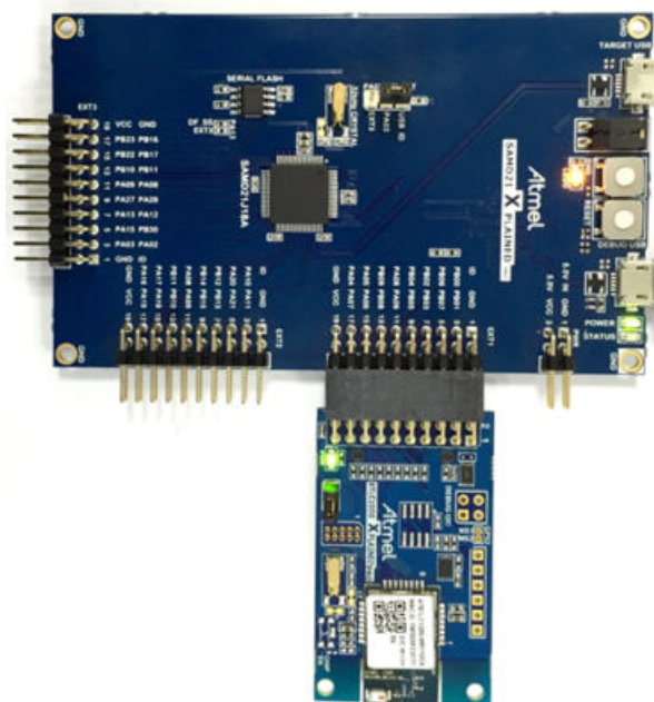
Figure 3-4. ATBTLC1000-MR Xplained Pro Extension Connected to the SAM D21 Xplained Pro
