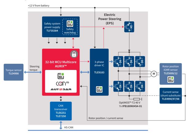
Thanks to its state-of-the-art safety features, the new TriCore™ AURIX™ family enables systems to achieve the highest ASIL-D safety level, which is already required in contemporary steering systems.
