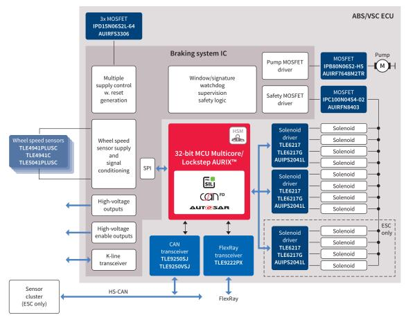
Thanks to its state-of-the-art safety features, the new TriCore<sup>™</sup> AURIX<sup>™</sup> family enables systems to achieve the highest ASIL-D safety level, which is already required in contemporary braking systems. The latest diverse lockstep technology with clock delay (diverse lockstep core) significantly reduces the software overhead and enables fast time-to-market. The scalability supports an optimized cost-performance fit for basic ABS systems up to highly integrated ESC systems.
