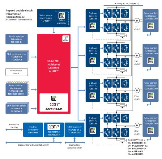
Thanks to its state-of-the-art safety features, the new TriCore<sup>™</sup> AURIX<sup>™</sup> family enables systems to achieve the highest safety level up to ASIL-D. The rich scalability of the AURIX<sup>™</sup> family permits a platform approach that meets the needs of a range of transmission systems. Furthermore, the hot temperature package and bare die solutions enable AURIX<sup>™</sup> to be used in both attached and integrated control units.
