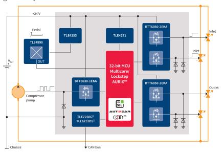
If ECU permanently supplied, you may need to add external protection against load dump 400 ms above 40 V.
