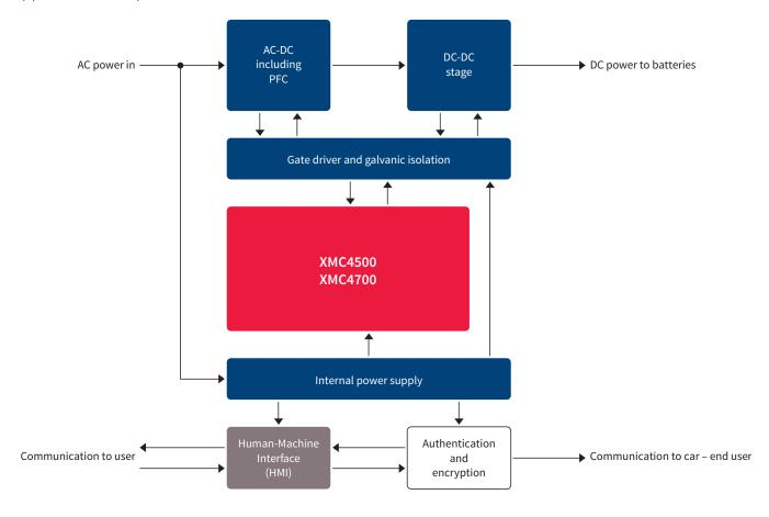
Off-board charging, where users can charge plug-in hybrids and pure EVs in private garages and open parking lots, demands an optimized solution with high MCU switching frequency to stay efficient and cost competitive. The Infineon XMC™ family is the answer!
