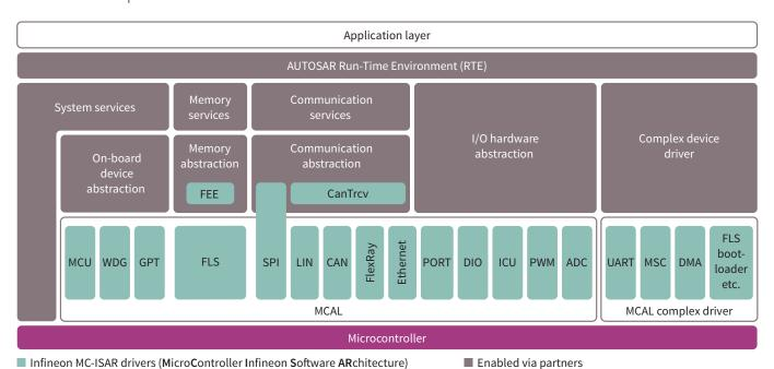
MC-ISAR MicroController – Infineon Software ARchitecture
