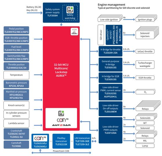
Thanks to its state-of-the-art safety features, the TriCore™ AURIX™ family enables systems to achieve the highest safety level up to ASIL-D. The scalable AURIX™ family includes the GTM, the de-facto industry standard timing module that supports highly complex engine management, while meeting the market's most stringent emissions regulations.
