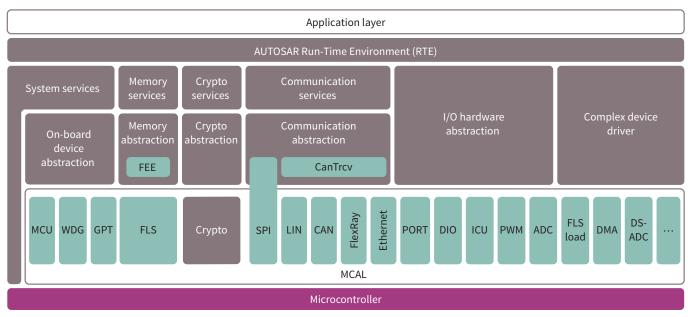
■ Infineon MC-ISAR drivers (MicroController Infineon Software ARchitecture)
