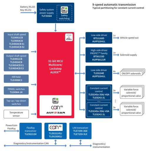
Thanks to its state-of-the-art safety features, the TriCore™ AURIX™ family enables systems to achieve the highest safety level up to ASIL-D. The rich scalability of the AURIX™ family permits a platform approach that meets the needs of a range of transmission systems. Furthermore, the hot temperature package and bare die solutions enable AURIX™ to be used in both attached and integrated control units.
