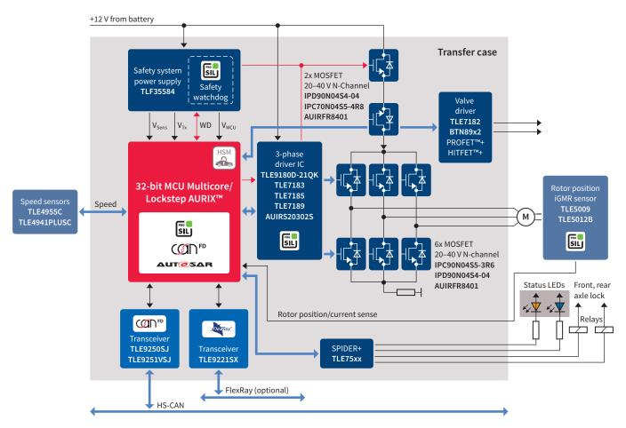
In Four-Wheel Drive (4WD) and All-Wheel Drive (AWD) vehicles, the transfer case is the part of the drivetrain responsible for the transfer of torque from the transmission to the front and rear wheels. The market now demands increased performance to drive BLDC motors and ever-greater functional safety requirements. AURIX™ has the state-of-the-art safety features required to enable systems to achieve ASIL-D, the highest safety level.
