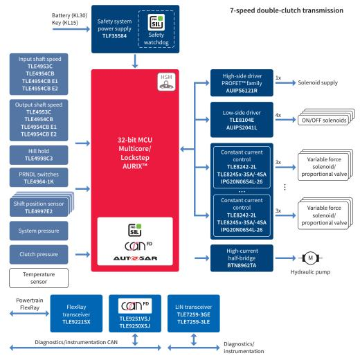
Thanks to its state-of-the-art safety features, the new TriCore™ AURIX™ family enables systems to achieve the highest safety level up to ASIL-D. The rich scalability of the AURIX™ family permits a platform approach that meets the needs of a range of transmission systems. Furthermore, the hot temperature package and bare die solutions enable AURIX™ to be used in both attached and integrated control units.
