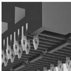
Staggered press-fit tails
