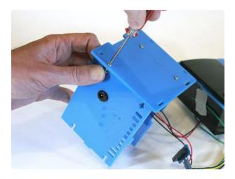
Connect the same side piece to the case back, using two nuts and screws as before.
