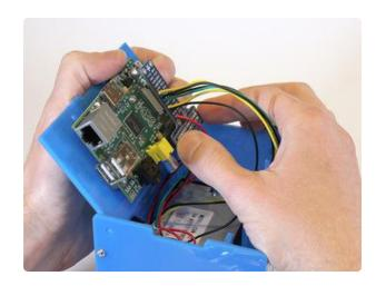
For the pre-2017 kit: Gently install the Cobbler board on to the Raspberry Pi GPIO header. Support the Pi board from below with the tips of your fingers...this prevents strain on the board and the case.
