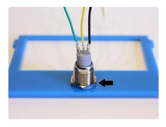
Fish the three wires through the button hole on the top case piece, press the button into place and secure with the included nut.
