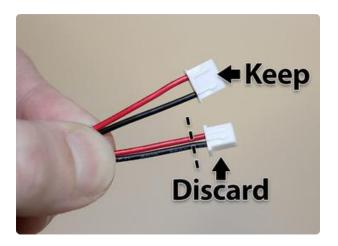
The power cable has a different connector at each end. We want to keep the wider of the two connectors for the printer. The small connector at the other end can be clipped off.
