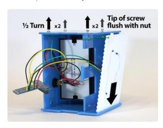
Slot one end of the front piece into the side of the case. The "torn receipt" effect should be at the bottom. There's no front or back to this piece, it can go either way, but Nimbus, our Internet of Things cloud mascot, wears his pompadour to the left.
