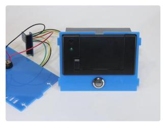
Being mindful of the wires and other attached components, slide the thermal printer through the large slot on the top case piece, with the feed button toward the BACK (the silver button is toward the front).
