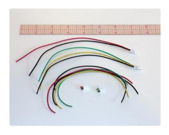
After cutting, you should have two cables, each about 7 inches long, both with a "wide" connector: one for power (red and black) and one for data (green, yellow and black).
