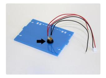
Secure the DC jack from the other side with the included nut. You'll need to fish the wires through this to get it into place.
