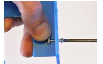
Use a screwdriver to turn the nut into place. Just "finger tight" is good for now... in subsequent steps we'll be loosening certain screws anyway.
