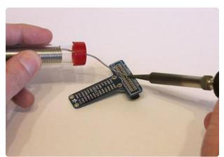
Tack the header in place by soldering just one pin (any will do) on the top side of the board. Notice we're soldering on the label side for this step.
