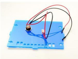
Fish the connector and wires through the DC hole on the <u>back</u> piece of the case (this the part with the etched Adafruit logo) and press the jack into place.
