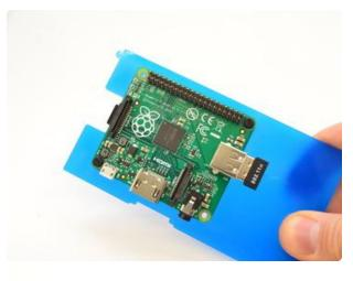
Push out the laser cut holes and mount the Raspberry Pi Board to the bottom plate using the included plastic #4-40 screws
