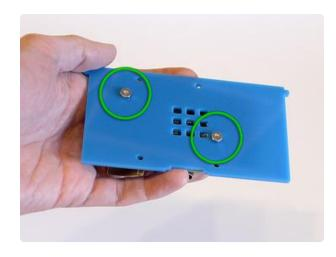
Position the bottom plate over the Raspberry Pi (remember, the scored side should face the board) and secure in place with two #4-40 nuts. Tighten the screws from the other side using a small screwdriver and gentle pressure — don't crank the screws down hard or you'll crack the case!
