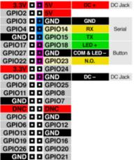
For the 2017-and-later kit, plug in the connections as shown here.
