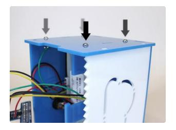
Tighten all four screws using a screwdriver (finger-tight).
