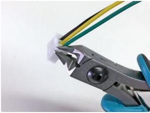
Use wire cutters to clip the side "wings" off the plug at one end of the data cable.
