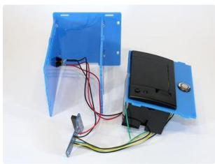
You should now have four nuts and screws installed in one side piece, holding the back and center support.
