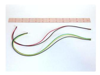
In the plastic baggie accompanying the thermal printer should be two cables, a bit over a foot long. The power cable has two conductors: red and black. The data cable has three conductors: green, yellow and black.
