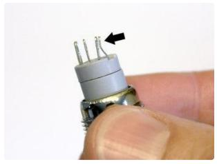
Using finger pressure or small pliers (gently!), smoosh the last two pins (COMMON and LED –) close together. We need to loop a single wire through both of them...
