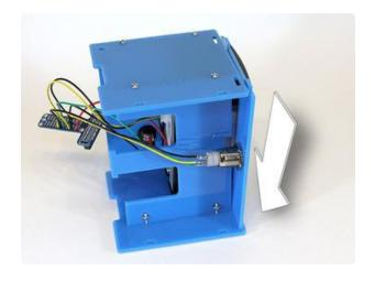
Slot one end of the top/printer piece into position. But with both sides in place, the slots at the other end are now blocked. The next few steps take care of all this...
