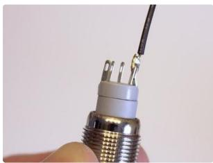
Loop the BLACK wire through the LED – and COMMON pins, bend it back on itself and solder.
