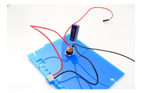
MAKE SURE THE NEGATIVE (shorter) LEG OF THE CAPACITOR IS CONNECTED TO BLACK/GND AND THE POSITIVE LED IS CONNECTED TO RED/5VDC.
