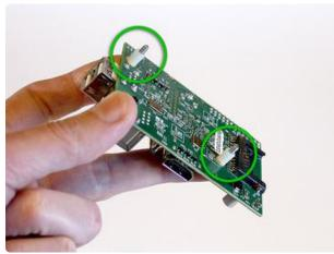
Using your fingertips to keep the screws in place, flip the board over and install a 1/4" nylon spacer over each of the two screws.
