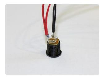
Repeat with the two black wires through the "outer" small leg (–).
