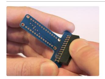
Normally the Cobbler would have a header soldered to the top, but we're doing something different with this kit: the socket sits on the underside of the board.
