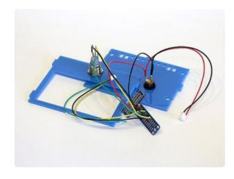
The button and power wires are now soldered to the Cobbler using the wiring diagram.
