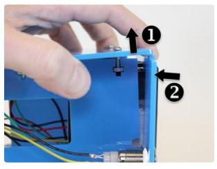
Lift the side of the edge piece. There should be just enough "play" for the tabs from the top piece to fit underneath.
