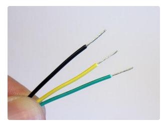
Strip about 3/8" of insulation from the end of three of the jumper wires: BLACK, YELLOW and GREEN. Twist the ends a bit to keep the strands from fraying.
