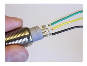
Repeat with the GREEN wire on the LED + pin and the YELLOW wire on the NO (Normally Open) pin.
