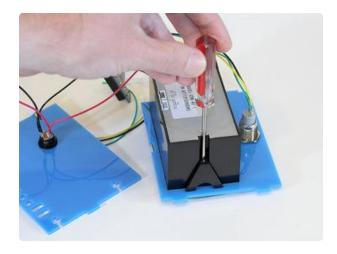
Set the printer and top piece face-down and insert the two brackets and screws. Use a small screwdriver to secure these in place. Use gentle pressure! Cranking these down tightly can crack the case.
