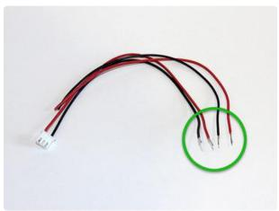
Strip about 1/4" insulation from the red and black wires on the power cable  $\underline{\text{and}}$  the spare wires.
