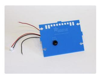
Fish the connector and wires through the DC hole on the <u>back</u> piece of the case (this the part with the etched Adafruit logo) and press the jack into place.
