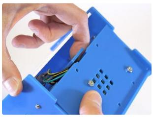
Carefully fold all the wires while swinging the bottom shut like a door. The center support piece has just enough flex to act as a latch.
