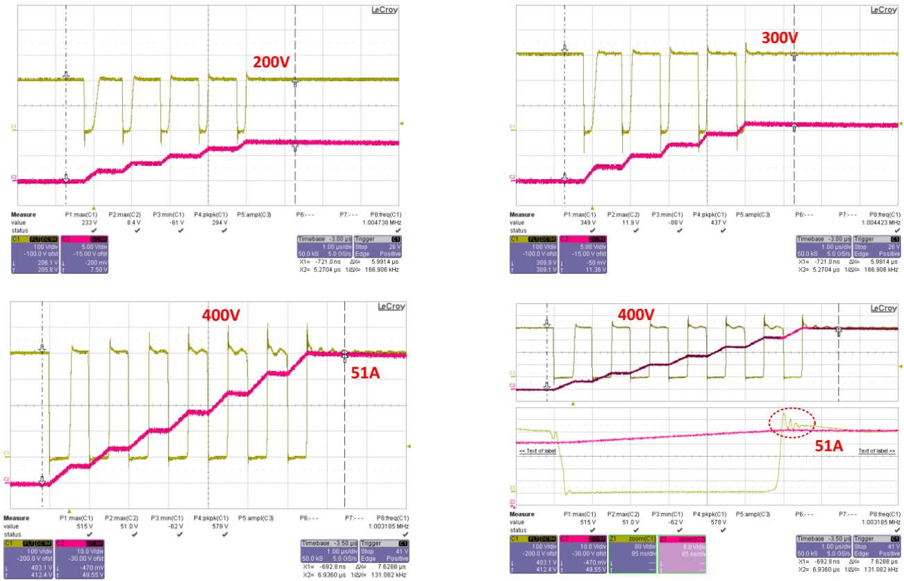
Figure 9. Low side switching waveforms: red = i_L , yellow = V_{ds}
