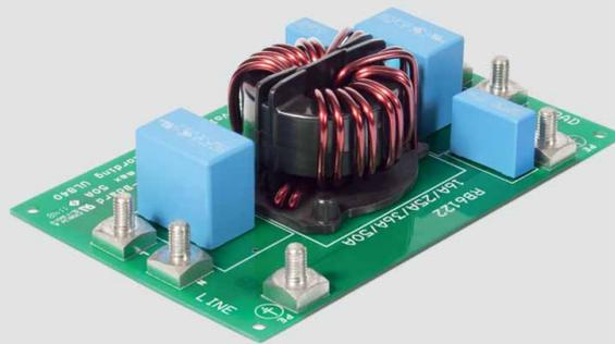
Fig. 8: Evaluation board for RB chokes
