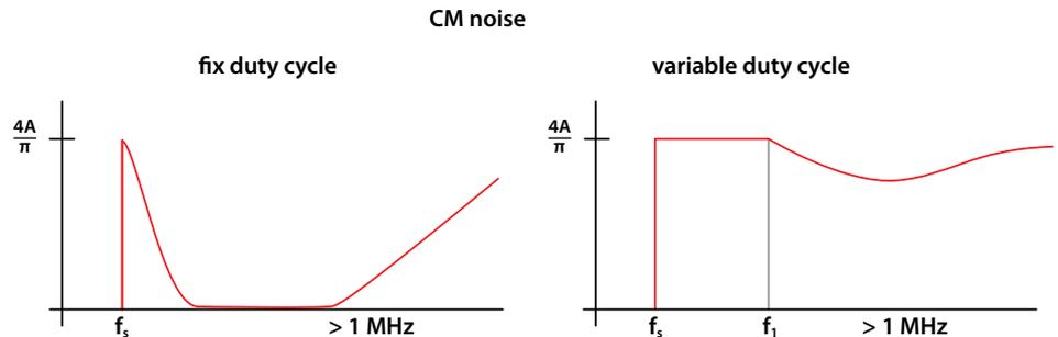
Fig.5: Simplified envelope curves of CM noise
