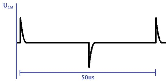
Fig. 4: Simplified CM noise signal
