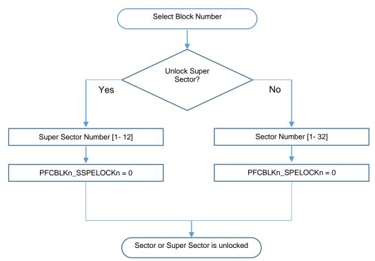
Figure 4. Unlock process for Sector or Super Sector
