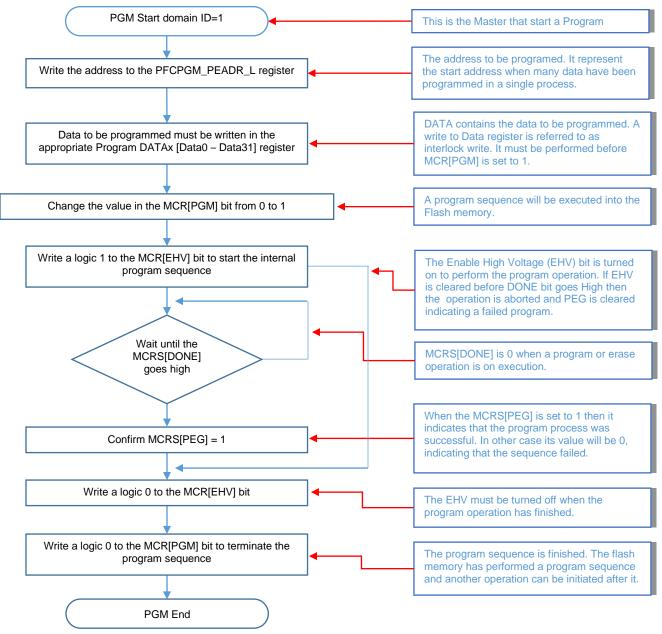
Figure 1. Program sequence flow diagram
