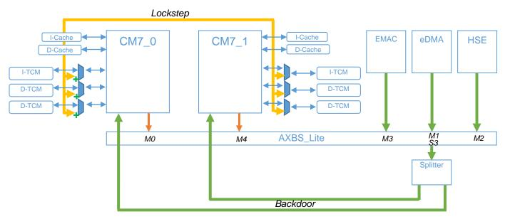
Figure 5. TCM memory accesses for S32K32x and S32K34x (Direct and Backdoor)
