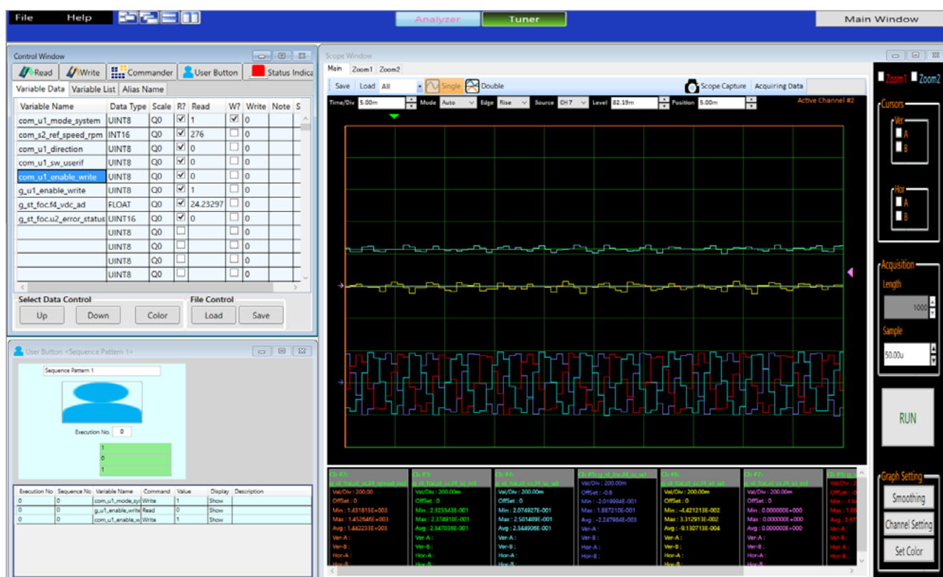
Figure 6-3: The Motor Control Workbench allows to auto-tune the parameters and to monitor the running system
