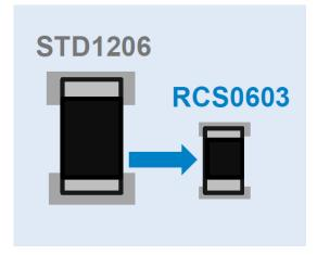
Also reduces total area of PCB that is occupied by resistors
