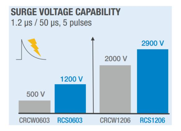
Single Pulse High Voltage Overload capabilities of RCS series parts also perform favorably compared to more standard thick film chip resistors. As shown in the chart above, which is considering a 1.2 $\mu$ s/50 $\mu$ s test condition, the RCS0603 series/size will withstand up to a whopping 1200V compared to the maximum of 500V that a standard thick film chip resistor of the same size while using resistance value 100k $\Omega$ .
