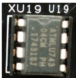
Figure 10. EEPROM in Socket
