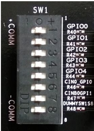
Figure 13. DIP Switch SW1
