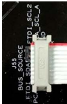
Figure 9. Aardvark Adapter Connection to J55
