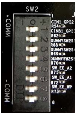
Figure 14. DIP Switch SW2
