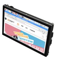
The Raspberry Pi LCD Touchscreen is designed with special holes on the back of the screen which makes it convenient to directly install the Raspberry Pi in the product. There is no need to provide external power for the touchscreen as the Raspberry Pi power supply is adopted.
