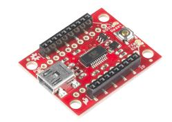
This Explorer USB board uses an FT231X USB-to-Serial converter that translates data between the computer and the XBee. The XBee Explorer USB offers a reset button, a
