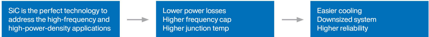
Figure 3: The deep-physics electrical characteristics of SiC ripple upward to yield tangible benefits for devices fabricated using that material and significantly affected system-level design issues. (Source: Mouser Electronics)
