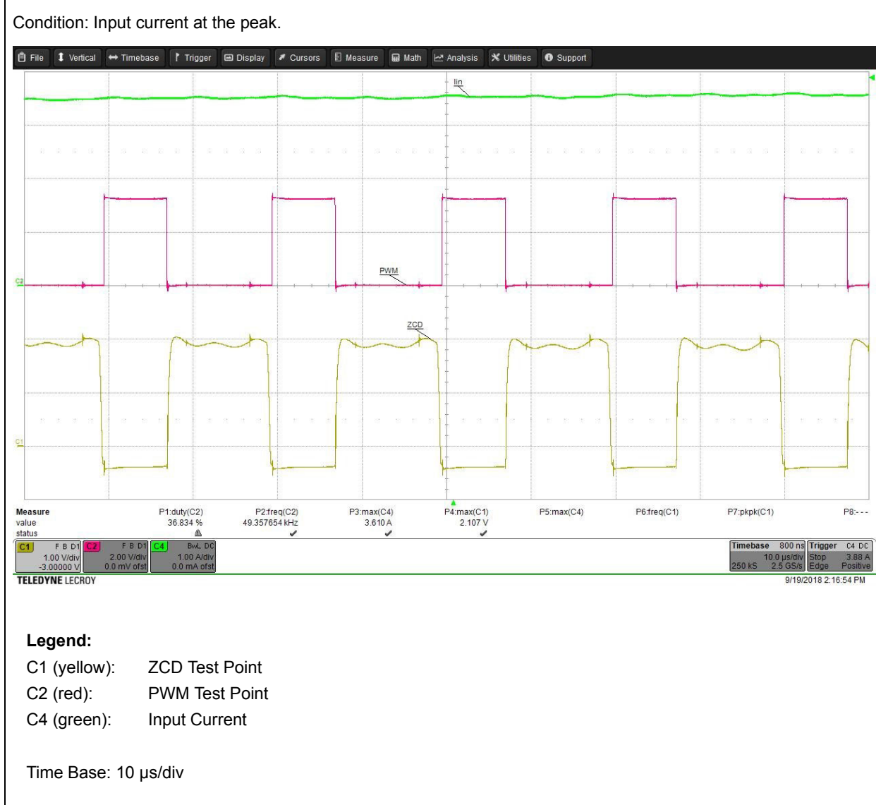
FIGURE 1-10: ZERO-CROSS DETECTION (ZCD), PWM TEST POINTS
