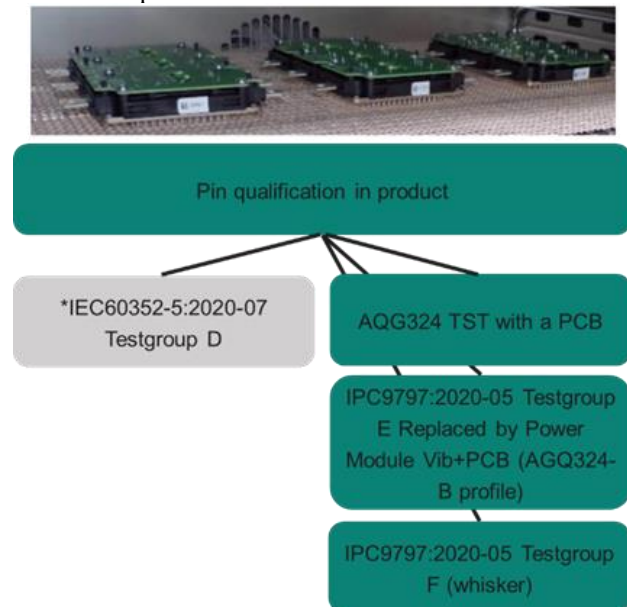
Figure 20 Pin qualification in the module
