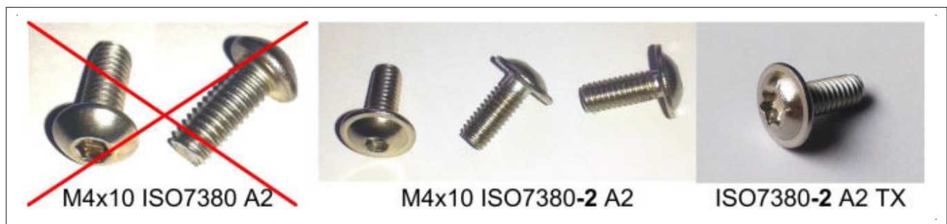
Figure 31 Picture of recommended screw type M4x10 ISO 7380-2 A2 (typical appearance). The correct type has -2 suffix to the ISO norm and is a screw with flattened round head (German: Linsen-Flanschkopfschraube). The recommended screw type is also available with a TX20 screw head: ISO 7380-2-A2-TX
