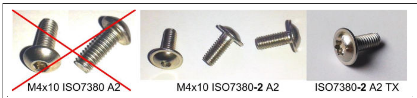
Figure 18 Picture of recommended screw type M4x10 ISO 7380-2 A2 (typical appearance). The correct type has -2 suffix to the ISO norm and is a screw with flattened round head (German: Linsen-Flanschkopfschraube). The recommended screw type is also available with a TX20 screw head: ISO 7380-2-A2-TX
