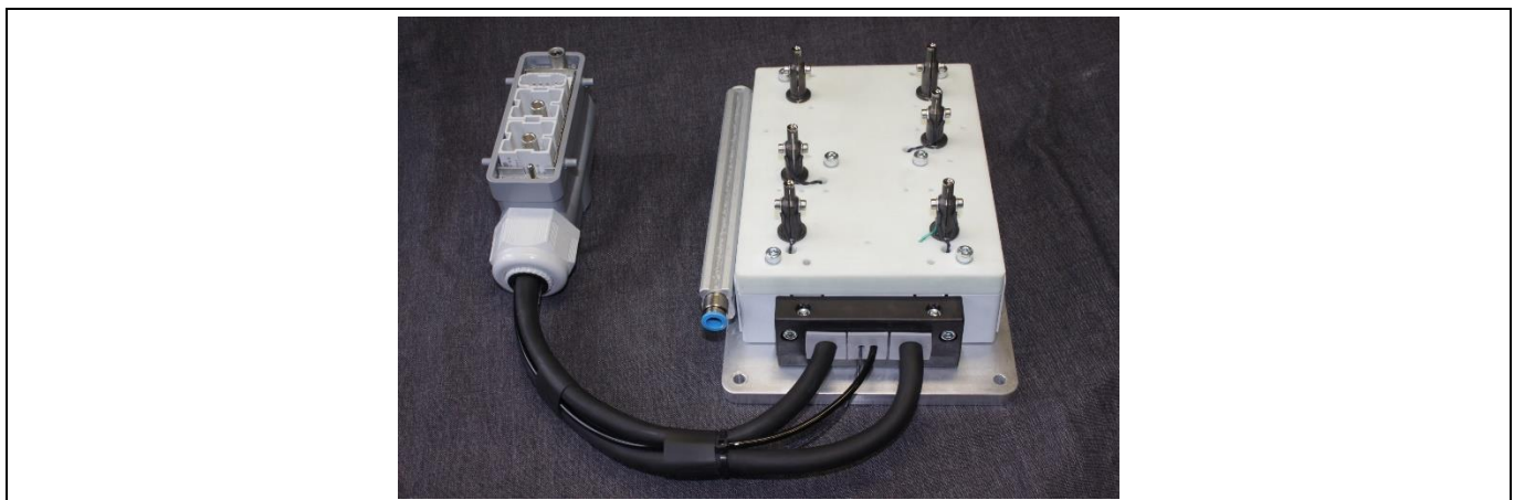
Figure 23 Tooling example for heat stake process of all six domes at the same time [8].
