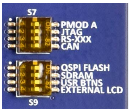
Figure 26. Function Select DIP Switches S7 and S9
