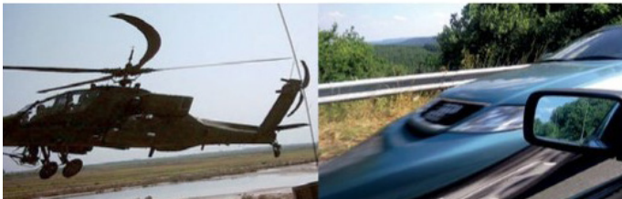
Figure 3: The rolling shutter effect. If the recorded objects are moving, strange motion artifacts might appear from sensors with rolling shutters.
