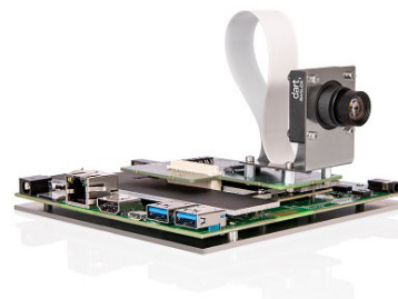
Figure 1: Embedded vision system consisting of Snapdragon 820 processing board and camera module with BCON for MIPI interface
