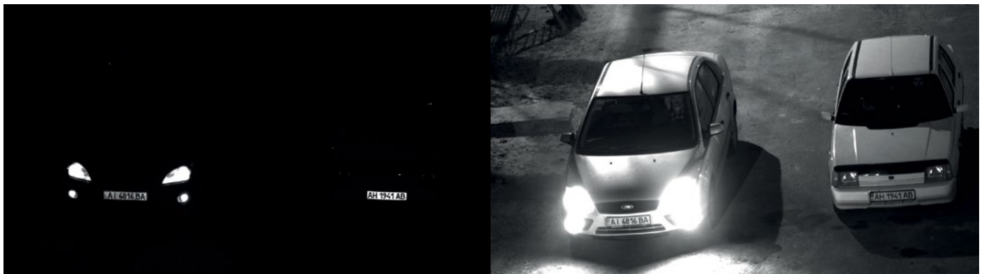
Figure 4: An example from Intelligent Traffic Systems (ITS): the image on the left was taken with a 4 tap CCD sensor, the KAI4050 Sensor from ON Semiconductor (formerly Kodak). The image on the right was taken with the new CMOS sensor IMX174 from Sony. In the image on the right, a clearly higher dynamic range can be seen very well as it allows for the driver as well as the license plate to be better recognizable in the same picture. Additionally, with nearly the same settings, the sensor is clearly more sensitive and there are correspondingly more details in the background.
