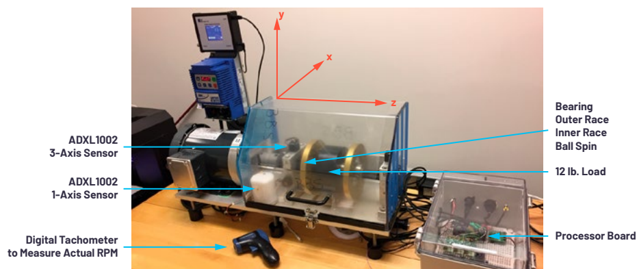
Figure 1. Channels X, Y, and Z measured vibration in the side-to-side, vertical, and fore-to-aft directions, respectively.
