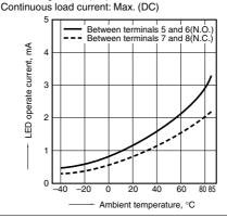
6. LED reverse current vs. ambient temperature characteristics
