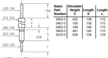
**Description:** 3400 - Double Tail Header Pin Packaging: Packaged in Bulk
