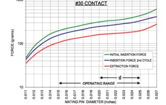
The insertion/extraction/normal force characteristics above were derived using a 30 microinch gold plated contact and polished steel gauge pins having a bullet-shaped tip.
