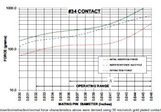
and polished steel gauge pins having a bullet-shaped tip.
