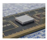
Tflex<sup>TM</sup> HD7.5 gap filler is a very soft silicone material in our high deflection series. With a thermal conductivity of 7.5W/ mk, Tflex<sup>TM</sup> HD7.5 is designed to provide superior pressure versus deflection characteristics. The material will provide minimal stress on components during application while maintaining low thermal resistance. As a result, less mechanical and thermal stresses will be experienced within your device.
