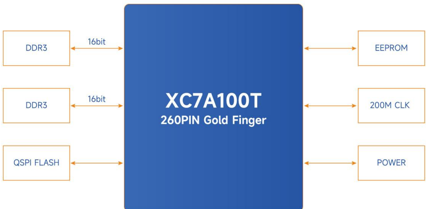
MYC-J7A100T Function Block Diagram
