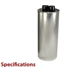
Type HV capacitors are constructed with low loss self healing metallized polypropylene film. Packaged in a cylindrical and oval metal cases. Type HV capacitors are ideal for AC filtering, CVT filtering/snubbering, line current reduction and voltage regulation in power supply applications.
