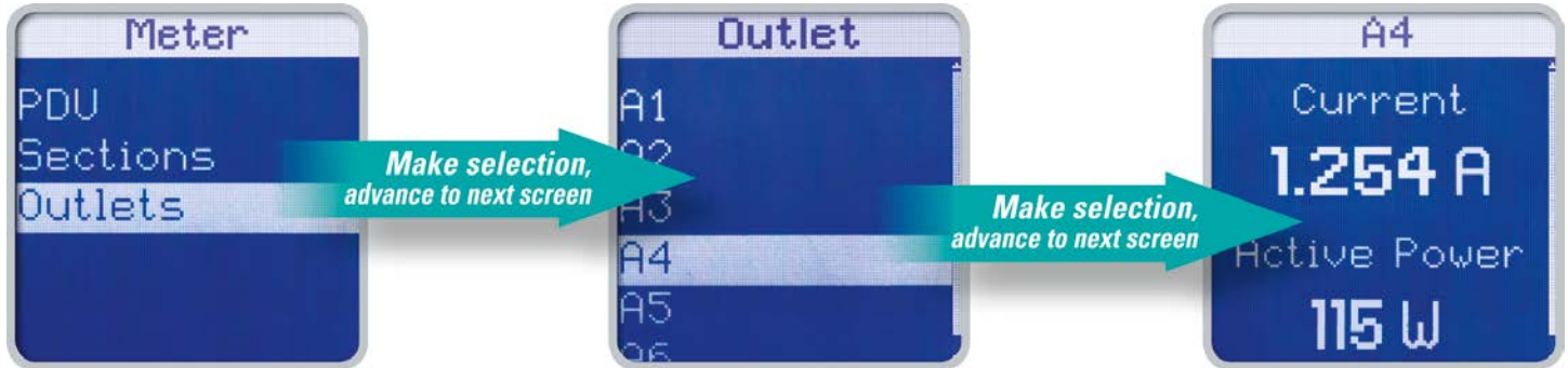
From meter screen, select outlets...
