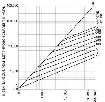
RMS SYMMETRICAL CURRENTS IN AMPERES A-B = ASYMMETRICAL AVAILABLE PEAK  $(2.3 \times \text{SYMM} \text{ RMS AMPS})$
