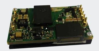
Advanced Energy's Artesyn AVQ200-36S12 series is a single output DC/DC converter with standard quarter-brick form factor and pin configuration. It delivers up to 19A output current with 12V output. Ultra-high 93% efficiency and excellent thermal performance makes it an ideal choice to supply power in telecom and datacom. It can operate over an ambient temperature range of -40°C ~ +85°C with air-cooling.
