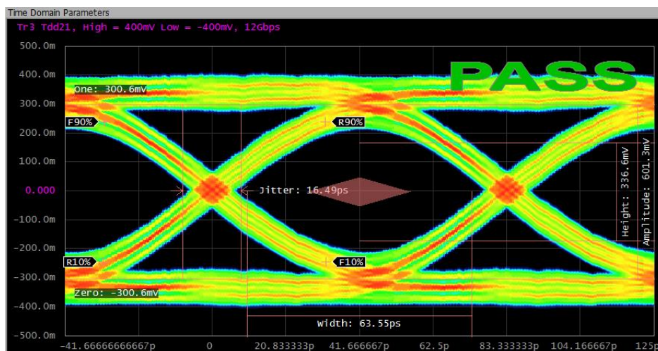
Figure 3. Data Rate 12Gb/s HDMI 2.1 Eye Diagram with SY205226DWC
