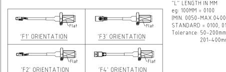
A = ASSEMBLED WITH CONNECTOR STANDARD = 0100, 0150, 0200) ORIENTATION OPTIONS: Tolerance: 50-200mm: ±5mm.
