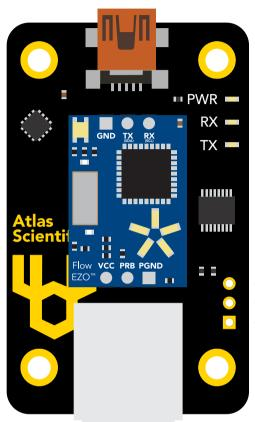
Connect Flow breakout board to the carrier board.
