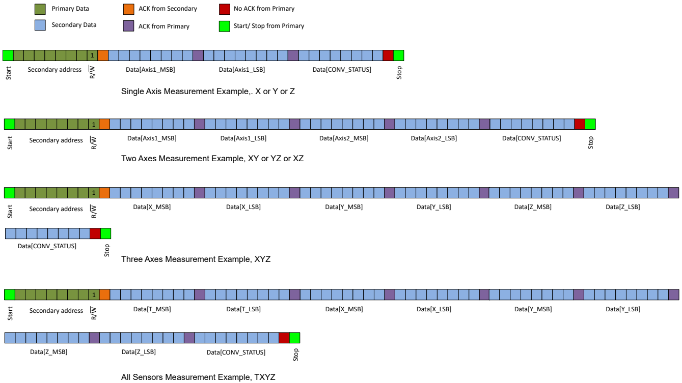
Figure 7-11. 1-Byte I 2 C Read Command for 16-Bit Data With CRC Disabled, CRC_EN = 0b
