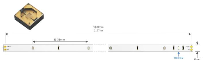
\*12 UVC LEDs applied per meter
