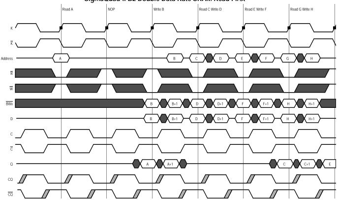
SigmaQuad-II B2 Double Data Rate SRAM Read First
