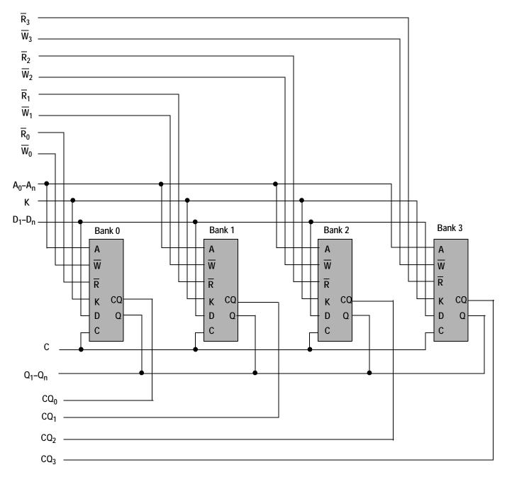
Example Four Bank Depth Expansion Schematic
