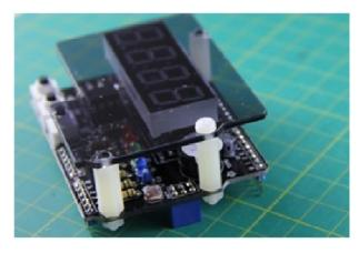
Tighten the standoffs with screws from the top.
