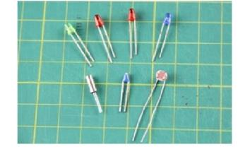
In the second row, from left to right, are a crystal, a thermistor and a light dependent resistor. They are not polarized, meaning it doesn't matter which way they are inserted into the board.
