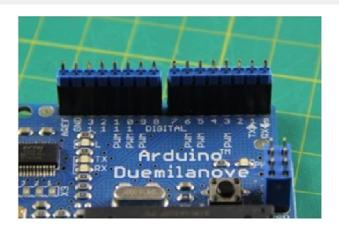
Insert all headers including the ISP header. Then stack the Tick Tock Shield on top.
