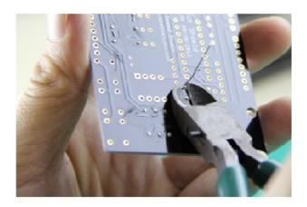
The directions above relay the basic technique for soldering. You can apply these steps when soldering the remaining components to the board. Now solder the remaining R3 lead and the other resistors. Preform them into U
