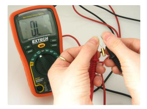
When pointing down, the switch is Open Loop (no continuity).
