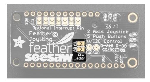
Because multiple featherwings of all kinds can be stacked, the I2C address can be changed if necessary. The Joy Featherwing's default I2C address is **0x49**, but soldering jumpers **A0** and/or **A1** can change this:
