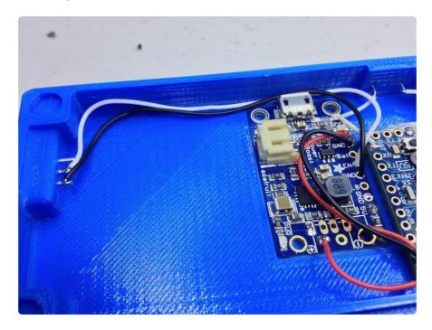
Now connect the EN and GND pins on the PowerBoost to the left and middle pins on the SPDT switch. Be sure to run the wires on the side instead of going straight to the switch. We want to leave some space for the LiPo battery.
