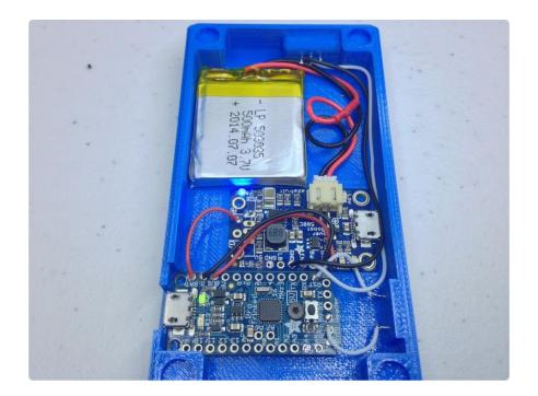
Finally we can connect the battery to the JST connector on the PowerBoost to test the circuit. If you slide the SPDT switch to the right, the boost converter will be enabled, and the system will power on. Make sure that you see both the blue LED on the PowerBoost and the green LED on the Pro Trinket light up.
