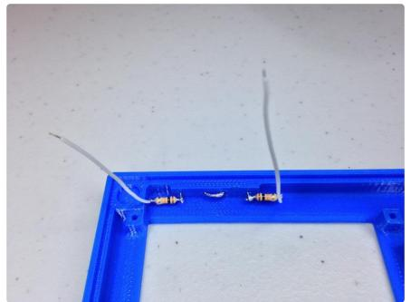
Then solder each of them to the outer two pins of the pushbuttons. The 4cm wire on the left,  $5 \, \text{cm}$  on the right.
