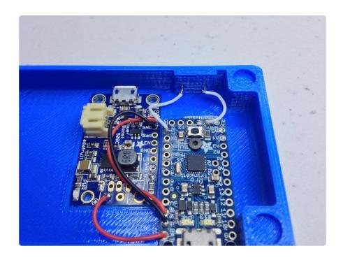
Then use two more short wires to connect the reset button to the Pro Trinket.
